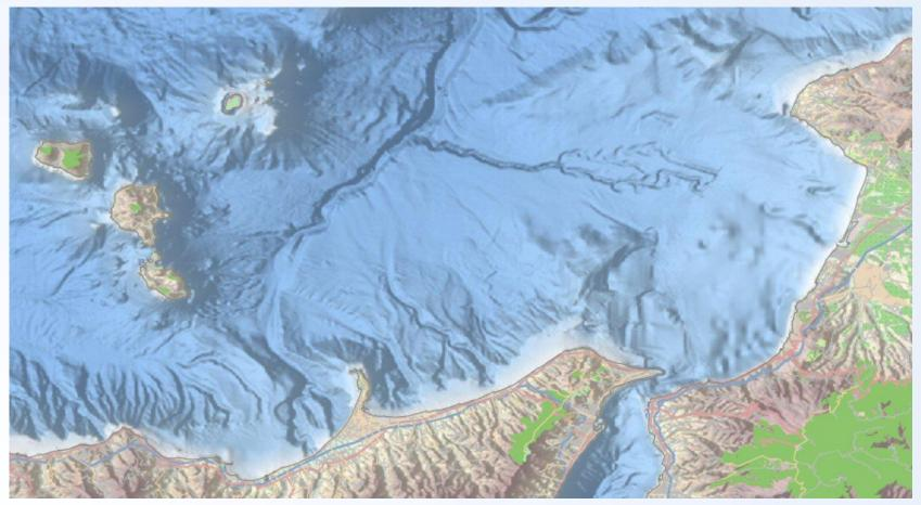
> 7000 survey data sets used to generate and provide a harmonized and higher resolution digital terrain model for all European seas – comparison with GEBCO
