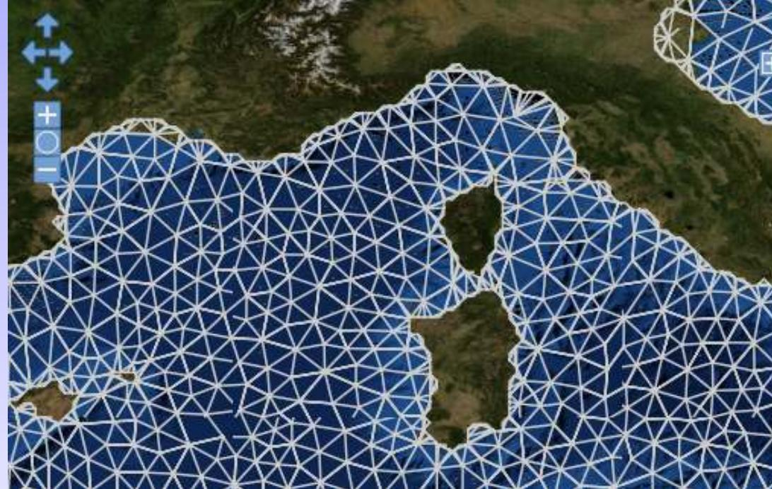
Solution by finite element method. Note decoupling of subbasins.
